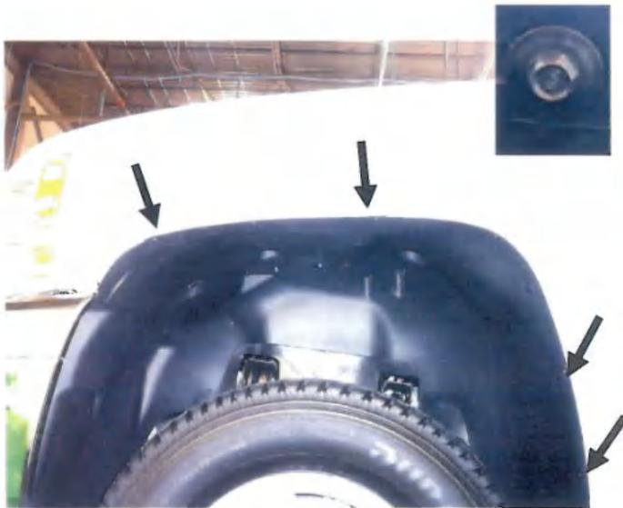
**STEP 4:** Place the Fender Flare on the vehicle into the position of best fit. Note where the slots in Fender Flare at positions A, B, C, and D align with the existing screws in the vehicle. Remove Fender Flare. Use the original manufacturer's hardware that is in the wheel arch of the vehicle to fit the Fender flares. Remove the x4 9/32" (7mm) socket head screws from the fasteners on the vehicle.
