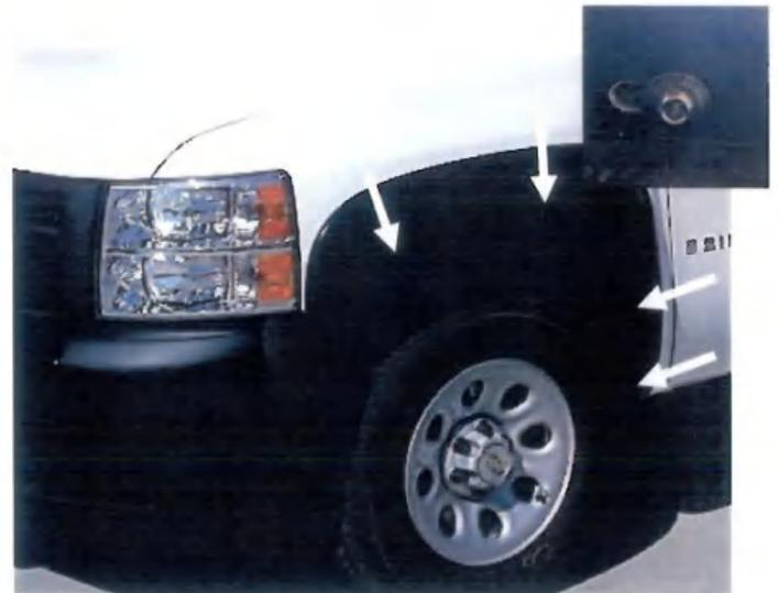
**STEP 5:** Place the front Fender Flares onto the vehicle and line up the holes on the part with screw holes on the vehicle. Re-Install the socket head screws into the fender to secure the Fender Flares. Fit the Fender Flares loosely until the Fender Flares are aligned as desired, when satisfied tighten the screws fully to ensure rubber seal is flush neatly against the body.
