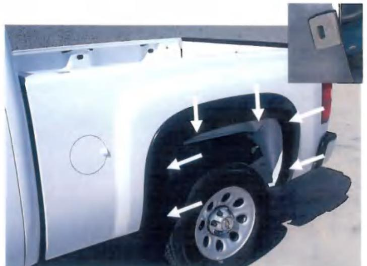
**STEP 9:** To secure the Fender Flare to the body, take the black metal clips and slide them over the Fender Flare and the inner wheel arch lip. Position the clip so that the barb in the clip locates in the slot of the Fender Flare. Ensure all fixing points are secure and that the rubber seal is flush neatly against the body.
