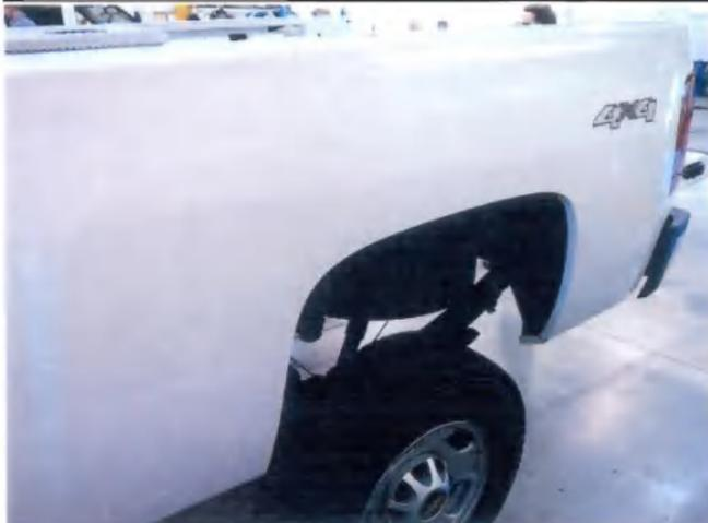
**STEP 8:** Clean the body areas where the Fender Flares will make contact. Ensure fenders are dry prior to install.
