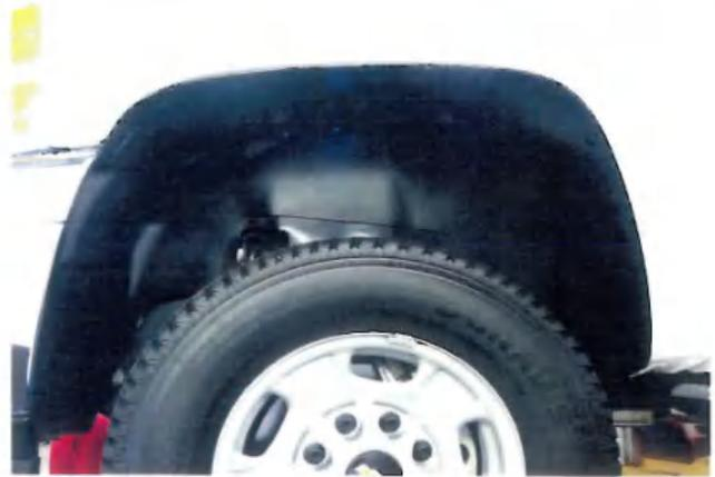
**STEP 3:** Clean the body areas where the Fender Flares will make contact. Ensure fenders are dry prior to install.
