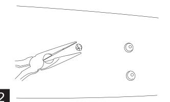
Install driver side rear motor linkage through this hole in frame.
