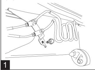
Disconnect brake lines from frame by squeezing outside of plastic fastener. CAUTION: Do not break plastic fastener. Disconnect <u>first</u> and <u>third</u> fastener from front.
