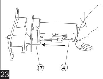
Slide rubber grommet on Wire Harness into slot of Motor Cover. Slide Motor Cover over Motor.
