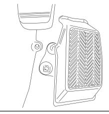
Pry up front door sill plates and remove kick panel fasteners and panels on driver and passenger side.
