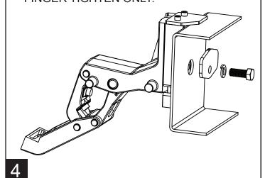
Install brake line stand-off inside driver rear frame rail as shown.
