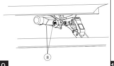
Secure controller to factory wire loom using supplied 11" wire ties. Connect Red fused wire to stud on battery positive terminal. Connect Black wire to ground on inner fender panel.
