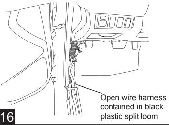
Install Single Diode Harness as shown on Pink/ Black wire (12 volt negative with door open) and connect to Power Step Pink/Black trigger wire. Make sure to install the diode toward the front of the vehicle.
