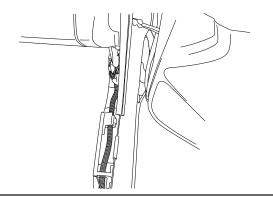
Connect Red/Black Power Step trigger wire to Red/Black factory Door Ajar signal wire (12 volt negative with door open) using supplied
