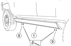
Torque linkage to frame through bolts from step 4 to 40 ft-lbs(54Nm)
