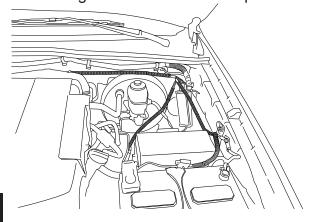
Torque 3/16" Allen bolts to 10ft-lbs. (13.5Nm)
