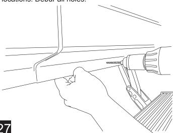
Insert grommet into drilled holes. Insert lamp wires through the grommets. (Silicon lube will help wires slip through grommets.)
