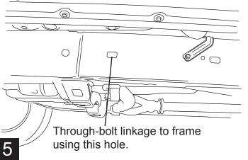
Secure Linkage Assembly to frame. FINGER TIGHTEN ONLY.
