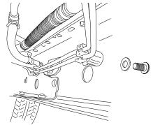
Replace all brake line fasteners.
