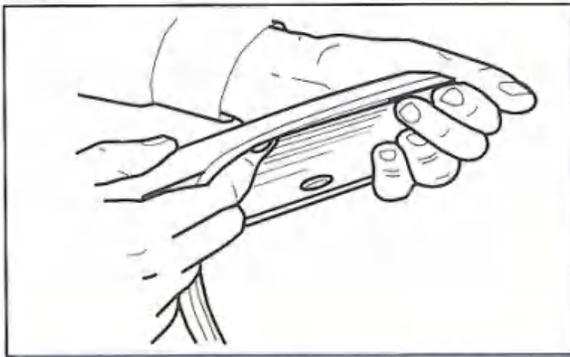
4. Remove approximately 2" (50mm) of the protective liner from the extrusion. Fit the extrusion to the Fender Flares along the edge that comes in contact with the vehicle's body panel, ensuring the double sided tape is being adhered to the inside surface of the fender
