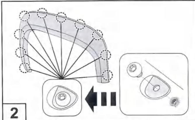
Attach 10 bolts to each Fender Flare using a 3/16" Allen key and a 1/2" wrench/socket.
