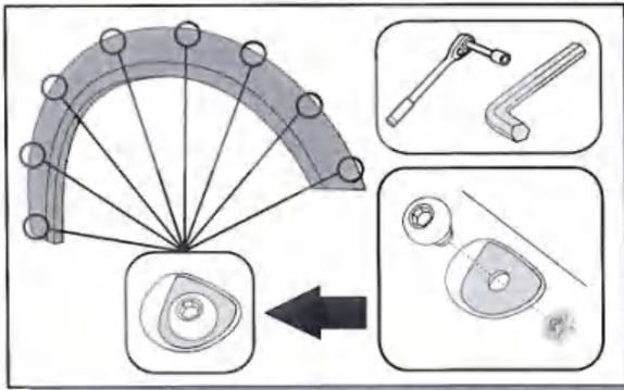
2. Attach bolts to each Fender Flare using a 3/16" Allen key and a 1/2" wrench/socket.
