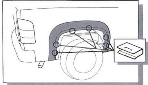
7. To secure the Fender Flare to the body, take the black metal clips and slide them over the Fender Flare and inner wheel arch lip. Position clip so that the barb in the clip locates in the slot in the Fender Flare. Ensure all fixing points are secure and that extrusion is flush neatly against the body.
