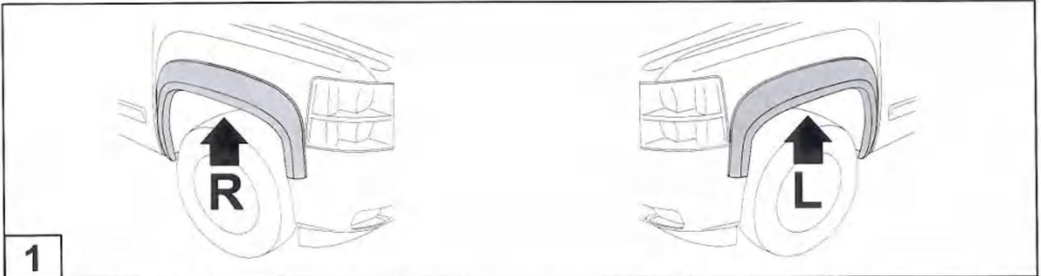
Ensure that both left and right hand Fender Flares suit the profile of the vehicle. Note the areas where the Fender Flares come in contact with the vehicle. **NOTE:** Before fitting Fender Flares remove any mouldings, strips or existing flares from the wheel arch. If there is a body side moulding, mark where the moulding is to be cut, alternatively the Fender Flares can be cut to go around the moulding. Be sure to allow enough room for the extrusion.
