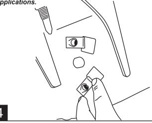
Offset the step pad forward and secure using provided PT Screws. Tighten to 5 ft-lbs using T25 torx bit. Note: Drivers side shown
