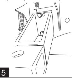
Adjust step pad to be in line with fender and torque bolts from Step 2 to 20ft-lbs.
