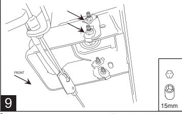
www.amp-research.com 2/3 IM75403 rev 03.31.16 For 2011 - up Short bed models: Remove the two rearmost u clips off the bracket and change orientation of the bolt so that the bolt head is on the outside of the bracket. Torque bolts to 16 ft-lbs.
