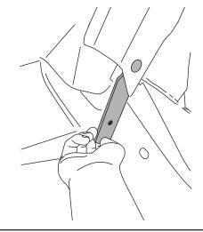
Locate the step pad on the center position of the lower linkage assembly and secure using provided PT Screws. Tighten to 5 ft-lbs using T25 Torx bit. Align Step pad to be in line with fender.
