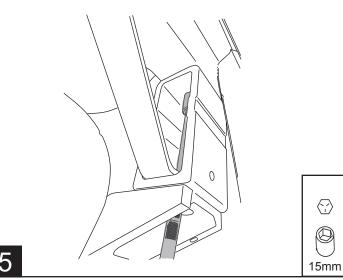
Using a 15mm socket with extension, align bolt with threaded plate. Torque to 20 ft-lbs.
