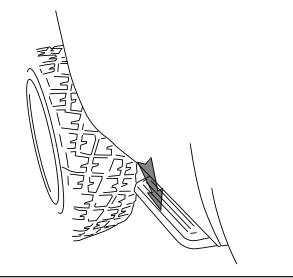
To retract, gently kick up on the underside of the step pad.
