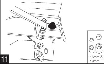
For all other Models: Attach bracket to threaded hole in frame mount. Rotate bracket into position and use the provided M12 hardware.
