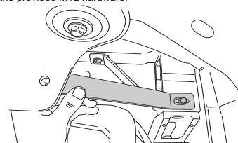
NOTE: If a hole is not provided on a factory body mount, a hole must be drilled using a 1/2" drill bit.
