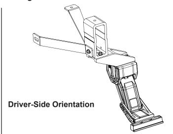
Using a 15mm Socket assemble Lateral mount onto Linkage assembly. Torque bolts to 20 ft-lbs. Note: Drivers side shown. Mirror for passenger side (See image in step 1 for passenger orientation).
