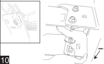
For 2011 - up Short bed models: Attach bracket to threaded hole in frame mount. Rotate bracket up to position and use provided M12 Hardware. Tighten M8 bolt to 16 ft-lbs and M12 bolt to 35 ft-lbs.
