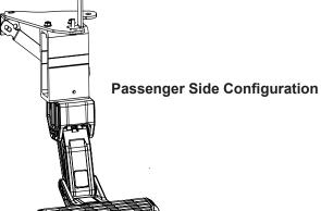
Using a 12mm socket or wrench loosen both brake cable brackets. **Note: Passenger side only has one bracket to remove.**
