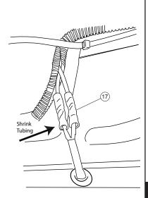
Close and wrap with conduit and electrical tape. Secure all loose wires with cable ties with lamp wires pulled upward to avoid any wire snagging.
