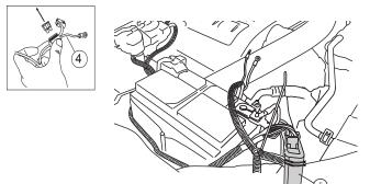
Attach wire harness to controller (make sure connector locking tabs fully engage). Mount controller with the two 11" tie wraps to factory conduit, just forward of battery.
