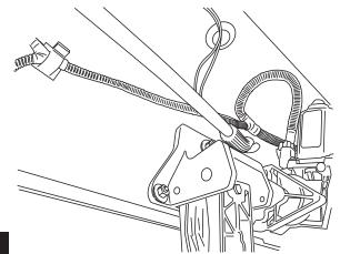
On Supercrew models, remove grommet in floor panel above front linkage on driver side. Poke small hole into grommet and thread the two trigger wires through and up into the cabin of vehicle. Seal grommet with silicone sealer.
