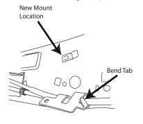
A. Remove bolt with 13mm box B. Remove and relocate J-Clip to location shown above. Bend bracket tab flat to reinstall.
