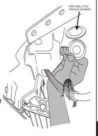
Connect red and black power leads to battery. Red lead goes to positive. Route shorter leg of harness down passenger-side wheel well and longer leg of harness down along driver side wheel well. Secure with tie wraps.
