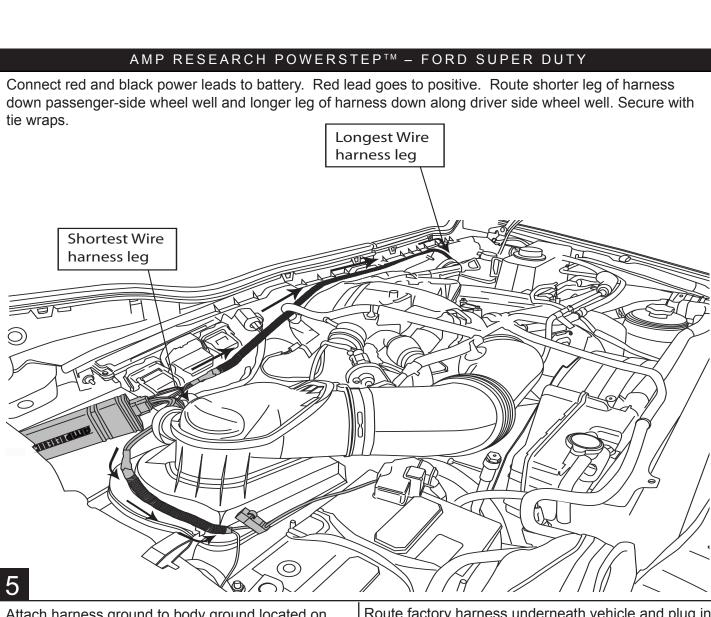
Attach harness ground to body ground located on inner fender.
