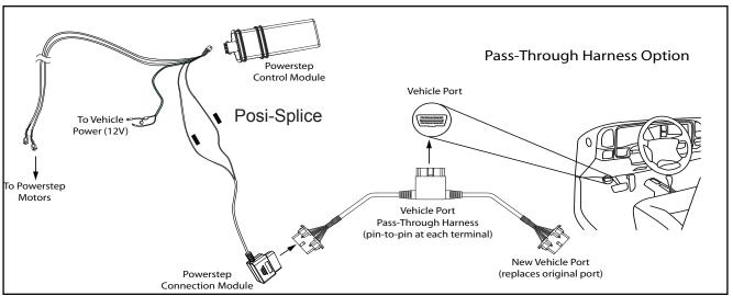
Wire OBD II connector with Posi-Splice.
