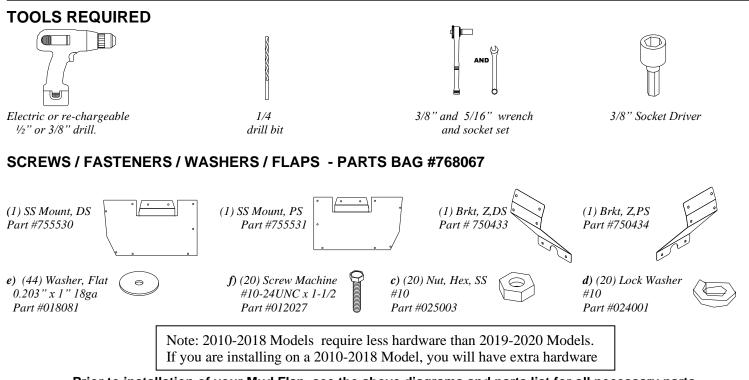
Prior to installation of your Mud Flap, see the above diagrams and parts list for all necessary parts. Start on the driver side.
