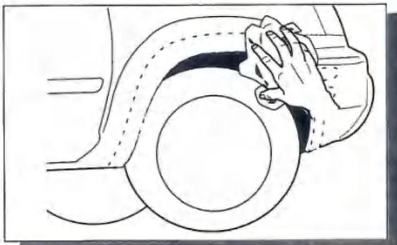
2. Wash the areas of contact on the vehicle and wipe dry both the vehicle and the Fender Flares with a clean cloth. Ensure inside of Fender Flares where extrusion is attached is clean, use alcohol wipe supplied to clean surface.
