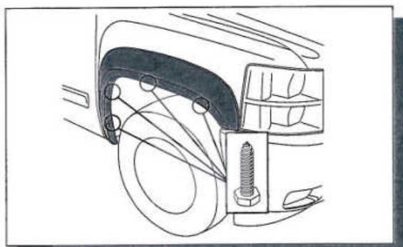
8. Re-Install the socket head screws into the fender to secure the Fender Flares. Fit the Fender Flares loosely until the Fender Flares are aligned as desired, when satisfied, tighten the screws fully and ensure extrusion is flush neatly against the body.
