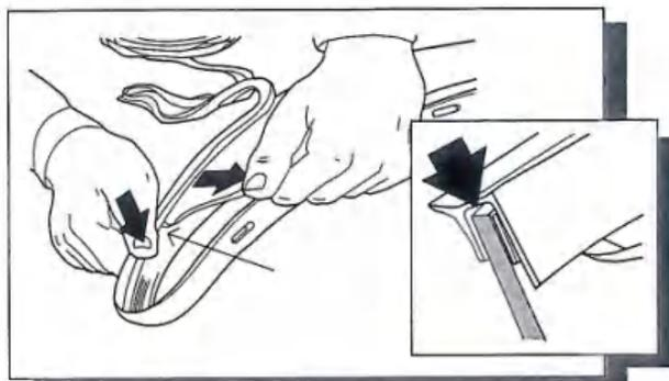
4. Pulling at right angles to the extrusion, remove the liner from the extrusion in small portions and apply thumb pressure to ensure that it adheres to the Fender Flares.
