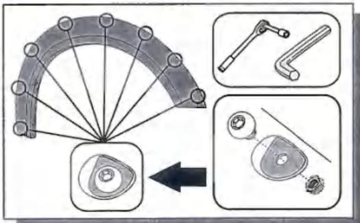
2. Attach 9 bolts to each Fender Flare using a 3/16" Allen key and a 1/2" wrench/socket. (socket wrench and Allen key not supplied)
