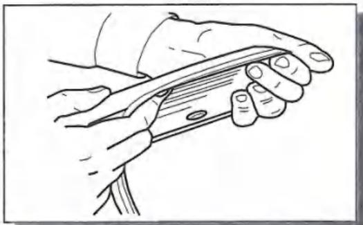
4. Remove approximately 2" (50mm) of the protective liner from the extrusion. Fit the extrusion to the Fender Flare along the edge that comes in contact with the vehicle's body panel.
