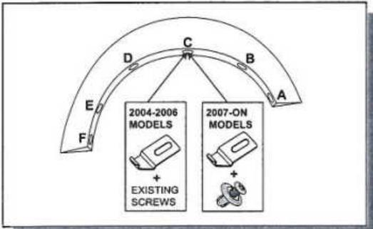
8. Note the correct hardware for position C (Right Fender Flare shown).
