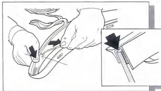
5. Pulling at right angles to the extrusion, remove the liner from the extrusion in small portions and apply
