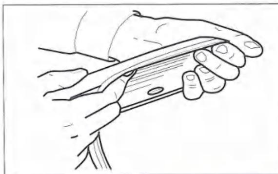
4. Remove approximately 2" (50mm) of the protective liner from the extrusion. Fit the extrusion to the Fender
