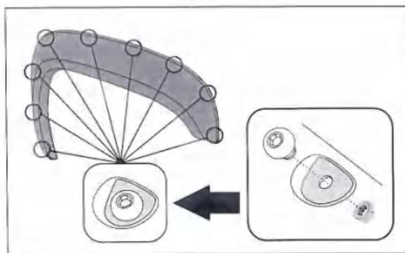
2. Attach 9 bolts to each Fender Flare using a 3/16" Allen key and a 1/2" wrench/socket.
