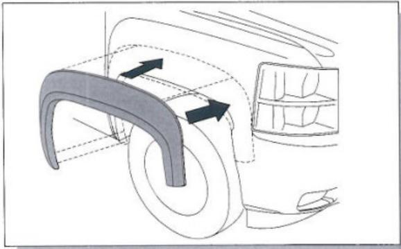
**8.** Place the front Fender Flares onto the vehicle and line up the holes on the part with the screw holes on the vehicle.
