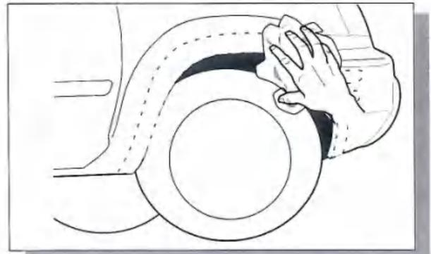
3. Wash the areas of contact on the vehicle and wipe dry both the vehicle and the Fender Flares with a clean cloth. Ensure inside of Fender Flares where extrusion is attached is clean, use alcohol wipe supplied to clean surface.
