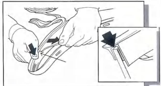
5. Pulling at right angles to the extrusion, remove the liner from the extrusion in small portions and apply thumb
