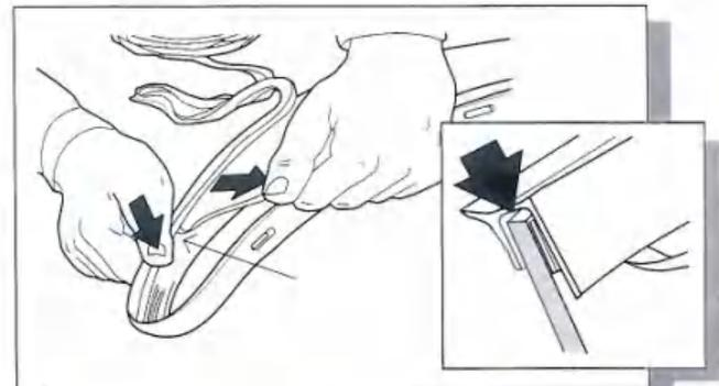
5. Pulling at right angles to the extrusion, remove the liner from the extrusion in small portions and apply
