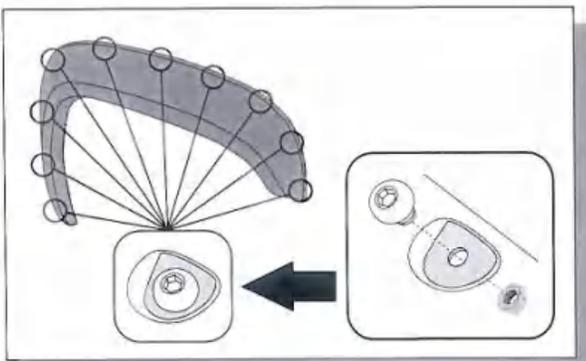
2. Attach 10 bolts to each Fender Flare using a 3/16" Allen key and a 1/2" wrench/socket.
