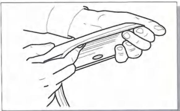
4. Remove approximately 2" (50mm) of the protective liner from the extrusion. Fit the extrusion to the Fender
