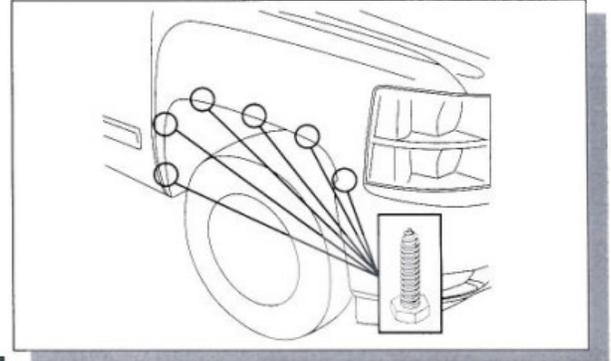
**7.** Use the original manufacturer's hardware that is in the wheel arch of the vehicle to fit the Fender Flares. Remove the 6x 7mm socket head screws from the fasteners on the vehicle.
