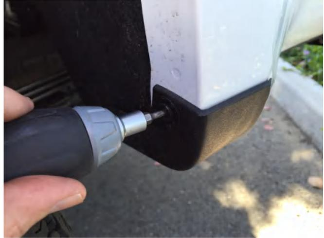
**STEP 11:** Using #15 Torx head screwdriver, remove lower screw from the rear factory deflector. Remove the top factory screw from the front rear deflector. Maintain screws for re-install.
