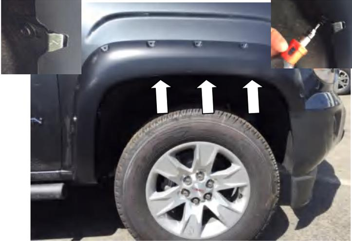
**STEP 7:** Place the Fender Flare onto the vehicle and fit into the correct position following the contours of the body. Use 3 of the retaining clips and previously removed factory screws to secure the Fender Flare to the body using #15 Torx head screwdriver. Make sure the clip securely engages the slots in Fender Flare.
