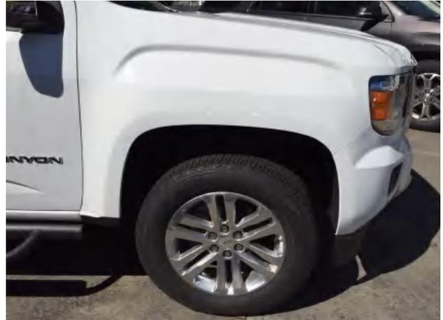
**STEP 4:** Clean the body areas where the Fender Flares will make contact. Ensure fenders are dry prior to install. Turning tires outward during install of each Fender Flare will ensure ease of install at bottom fixing points.
