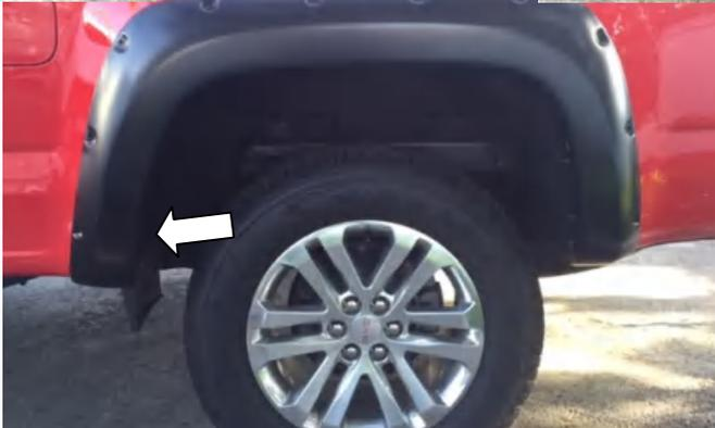
**STEP 12:** Place Fender Flare on the vehicle into the position of best fit, slide the bottom front end of Fender Flare between the existing mud flap deflector and wheel arch molding so that the slot in the Fender Flare is under the vacant hole in the mud flap. Using #15 Torx head screwdriver, loosely re-install the previously removed screw from front factory deflector.
