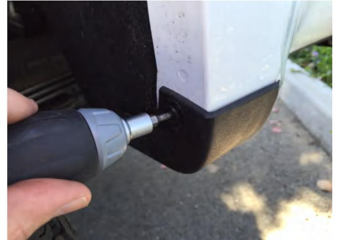
**STEP 6:** Using a #15 Torx head screwdriver remove bottom rear wheel arch molding screw. Maintain screws for re-install.
