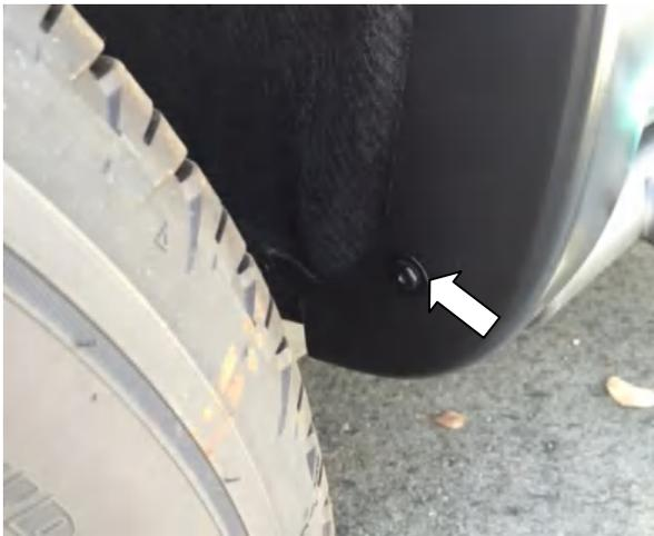
**STEP 9:** Loosely re-install previously removed factory screw through the slot in the Fender Flare at the bottom rear wheel arch using #15 Torx head screwdriver. Ensure Fender Flare is centered and in position of best fit on fender. Tighten all front fender fixing points to ensure a tight and secure fit. Ensure that the rubber seal is flush neatly against the vehicle body.
