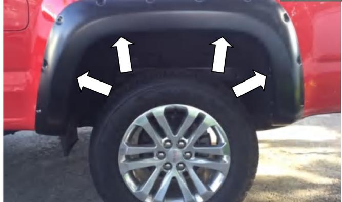
**STEP 13:** Install the provided U shape metal clips at the (4) remaining slot locations in the Fender Flare. Ensure that positive pressure is applied on the Fender Flare to the vehicle fender when installing clips. Slide the clips over the Fender Flare and the inner lip of the wheel arch molding ensuring that the barb in the clip locates in the slot of the Fender Flare.
