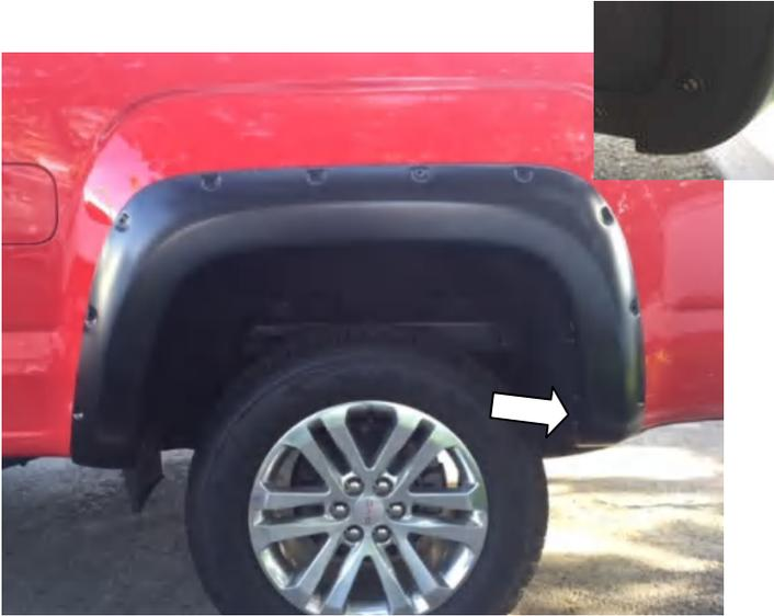
**STEP 14:** Using #15 Torx head screwdriver, re-install the previously removed screw through the bottom rear slot in Fender Flare and factory deflector. Ensure all fixing points are tight and secure and that the rubber seal is flush neatly against the vehicle body and factory deflector.
