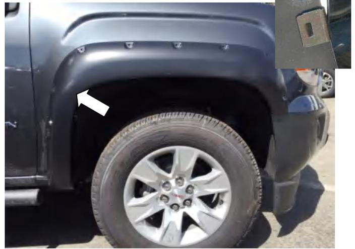
**STEP 8:** Install the provided U shape metal clip at the (1) remaining slot location in the Fender Flare. Ensure that positive pressure is applied on the Fender Flare to the vehicle fender when installing clips. Slide the clip over the Fender Flare and the inner lip of the wheel arch molding ensuring that the barb in the clip locates in the slot of the Fender Flare.
