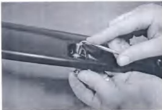
**STEP 1:** Attach the 11 bolts and nuts to each Fender Flare using a 3/16" Allen key and a 1/2" wrench/socket. (wrench /socket and Allen key not supplied). Ensure inside of Fender Flares where the rubber seal is attached is clean, using the alcohol wipes provided. Wipe away any residue with a dry clean cloth.
