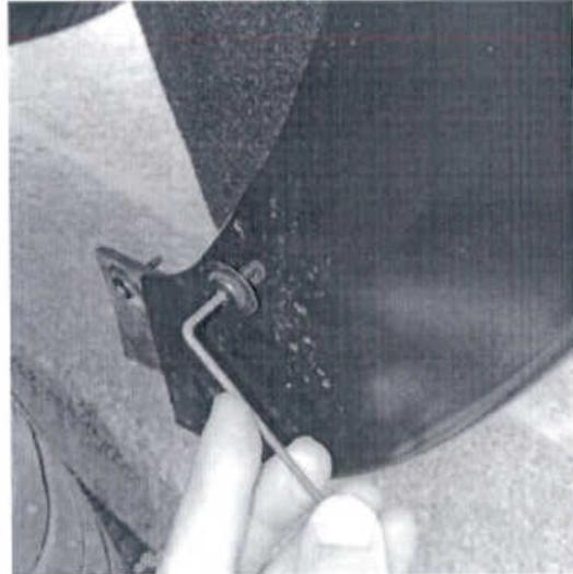
**STEP 8:** Using #15 Torx head screwdriver re-install the upper screw from the rear factory mudguard through the slot in the Fender Flare.
