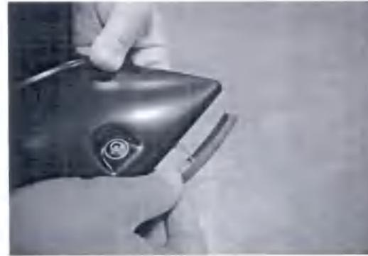
**STEP 2:** Attach the included rubber seal to the Fender Flares. Peel back 2" of the adhesive backing and position on the Fender Flare. Attach the seal to the Fender Flare, peeling back a few inches at a time. Ensure pressure is used to secure rubber seal to Fender Flare edge. Attach rubber seal along all areas the Fender Flare will make contact with the vehicle body. Trim excess rubber seal.
