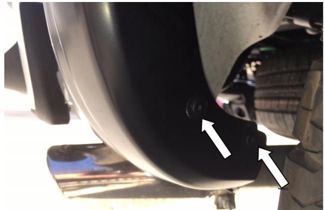
**STEP 15:** Place Fender Flare on the vehicle into the position of best fit. Note where the slots in Fender Flare align with the previously removed factory screws in the front and rear spats. Peel back 2 inches of the red tape liner on the fender flare extrusion at both ends, ensure liner is on the outside of part ref to step 18. Using #15 Torx head screwdriver re-install the upper and lower screws from the rear factory spat through the slots in the Fender Flare.
