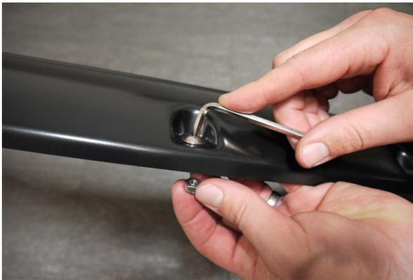
**STEP 10:** Attach the bolts and nuts to each Fender Flare using 3/16" Allen key/Trox and a 1/2" wrench/socket. (wrench /socket and Allen key not supplied). Ensure inside of Fender Flares where the rubber seal is attached is clean, using the alcohol wipes provided. Wipe away any residue with a dry clean cloth.
