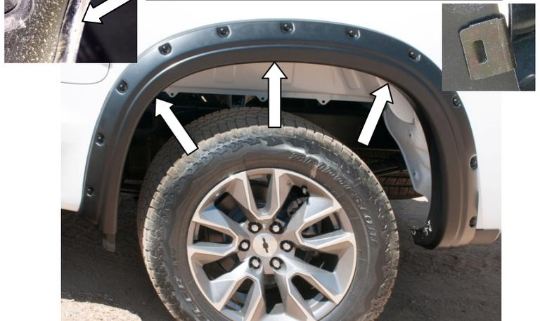
**STEP 17:** To secure the Fender Flare to the body, apply upward tension on Fender Flare to the vehicle fender when installing the black metal clips. Slide the clips over the Fender Flare and the inner wheel arch lip in the three locations shown. Position the clip so that the barb in the clip locates in the slot of the Fender Flare. Ensure all fixing points are tight and secure and that the extrusion is flush neatly against the vehicle body. Repeat install steps for the opposite side.
