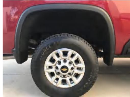
**STEP 15:** Place Fender Flare on the vehicle into the position of best fit. Note where the slots in Fender Flare align with the previously removed factory screws in the front and rear spats. Using #15 Torx head screwdriver re-install the upper and lower screws from the rear factory spat through the slots in the Fender Flare.
