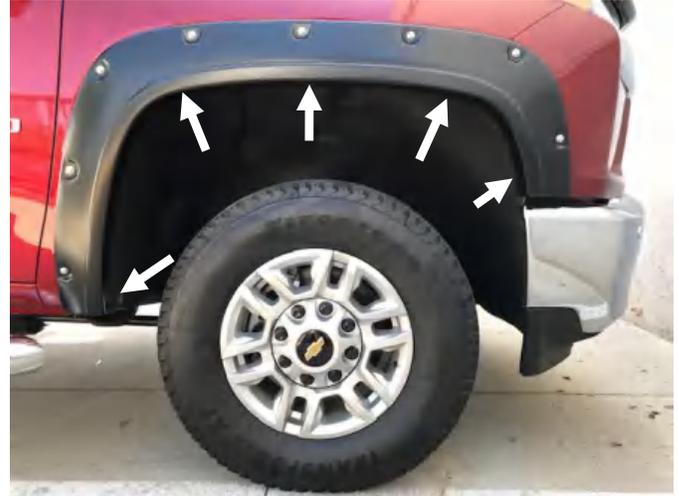
**STEP 7:** Place Fender Flare on the vehicle into the position of best fit. Using #15 Torx head screwdriver re-install previously removed factory mudguard screws at the upper and lower screw locations through the slots in the Fender Flare at the two noted locations. At the noted **C, D** positions secure the Fender Flare to the wheel arch by ensuring the notch in clip locates securely into the slot in the Fender Flare.
