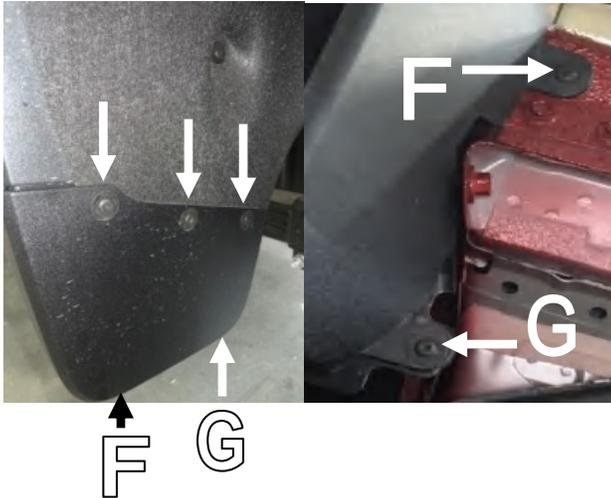
**STEP 14:** Using #15 Torx head screwdriver remove the two bottom screws from the rear factory spat. Maintain screws for re-install.
