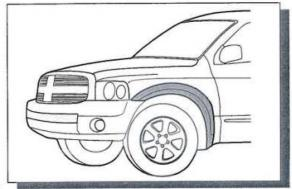
7. Fit the Fender Flare and align it with the existing screw positions. Secure the Fender Flare to vehicle by replacing the existing screws.
