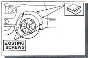
Note the correct hardware and existing screws position as shown. Also note the clips position.
