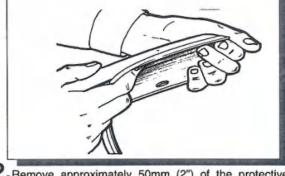
2. Remove approximately 50mm (2") of the protective liner from the extrusion. Fit the extrusion to the Fender Flare along the edge that comes in contact with the vehicles body panel.
