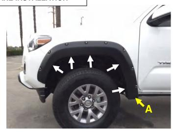
STEP 5: Hold Fender Flare on the vehicle in the position of best fit. For models <u>with</u> factory installed Fender Flares, note where above marked holes in Fender Flare align with existing screws in the vehicle. Make special note of "A". Remove the EGR Fender Flare and remove the (5) above indicated screws from the factory flare with a 10mm socket. <u>DO NOT</u> remove the factory flare, the EGR Fender Flare installs directly over the factory flare.
