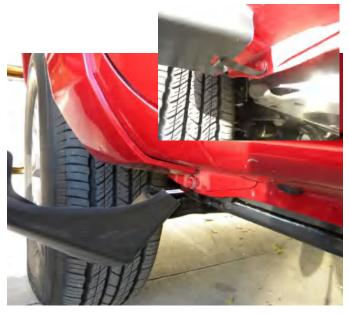
**STEP 9:** Begin installation by engaging the hook end of the clip into the slot in the bottom of the Fender Flare and begin rotating the Fender Flare vertically up to its position of best fit.
