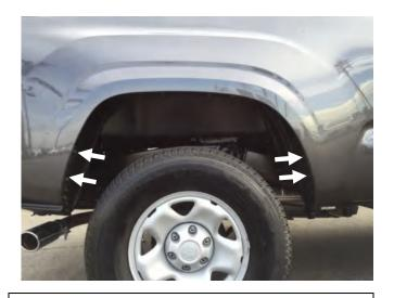
**STEP 15:** For models <u>without</u> factory installed Fender Flares, remove <u>only</u> the first (4) above indicated screws, from top to bottom of the fender, (2) each side, with a 10mm socket and retain for later re-installation.
