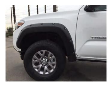
**STEP 12:** If necessary, make minor adjustments to the flares position to achieve the best fit for your vehicle and to ensure that the rubber seal is sitting flat against the painted vehicle surface. When satisfied fully tighten all (5) screw locations, in the above order in which they were just installed. Repeat install for opposite side.
