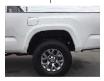
**STEP 13:** Clean the vehicle body areas with a mild soap and water solution, where the Fender Flares will make contact. Ensure fenders are dry prior to install.
