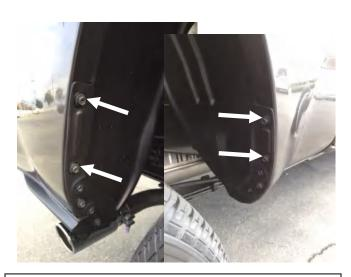
**STEP 15a:** Remove **ONLY** these (4) above indicated screws as mentioned in previous STEP 15, with a 10mm socket for models <u>without</u> factory installed Fender Flares. Leave all other remaining screws in wheel liner area. EGR Fender Flare will install directly over the remaining screws.
