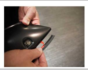
**STEP 2:** Attach the included rubber seal to the Fender Flares along the top leading edge where the Flare will make contact with the vehicle body. Peel back 2" of the adhesive backing and **apply the double sided tape to the inside surface of the Fender Flare**, peeling back a few inches at a time and applying pressure to secure rubber seal to Fender Flare.
