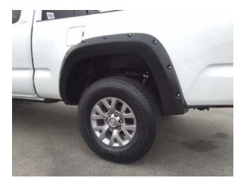
**STEP 18:** Remove remaining Hooked end Short Clip from hardware kit. Remove 10mm screw from previously noted area "A" in STEP 14 that aligns with mounting slot in Fender Flare. Install hook end of short clip into Fender Flare as shown above and re-install 10mm screw.
