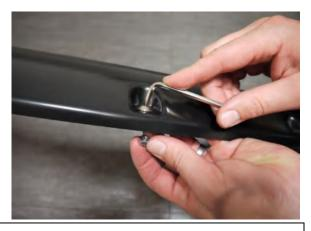
**STEP 1:** Attach bolts and nuts to each Fender Flare using a 3/16" Allen key and a 10mm wrench/socket (wrench /socket and Allen key not supplied).
