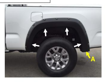
**STEP 14:** Hold Fender Flare on vehicle in the position of best fit. For models <u>with</u> factory installed Fender Flares, note where above marked holes in Fender Flare align with existing screws in the vehicle. Make special note of "A". Remove the EGR Fender Flare and remove the (4) above indicated screws from the factory flare with a 10mm socket. <u>DO NOT</u> remove the factory flare, the EGR Fender Flare installs directly over the factory flare.
