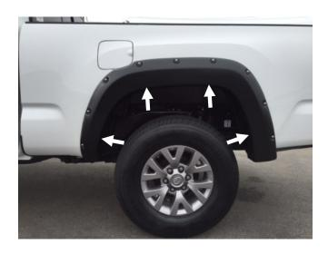
**STEP 16:** The protective plastic stone guard / wind splitter is different between with and without factory installed Fender Flare vehicles, it is necessary to hand file an additional approx. 1/4" out of the above indicted tip area of the Fender Flare cut-out to allow the Fender Flare to properly seat against the vehicle painted surface.
