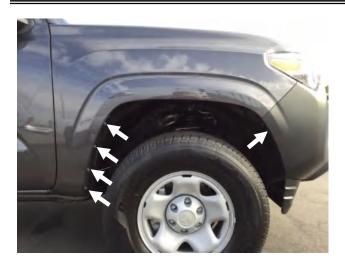
**STEP 6:** For models <u>without</u> factory installed Fender Flares, remove the (5) above indicated screws from the wheel liner with a 10mm socket and retain for later reinstallation.
