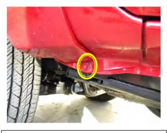
**STEP 7:** Again using a 10mm socket, remove the screw from the body sheet metal join referenced in STEP 5 as Special Note area "A" and retain for later re-installation.
