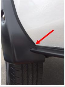
**IMPORTANT NOTE:** For rear area of rear Fender Flare. Trim rubber seal to initial contact edge of protective plastic stone guard / wind splitter attached to vehicle. **DO NOT** install rubber trim past this detail area. (Refer to above image)
