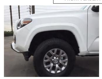
**STEP 4:** Clean the vehicle body areas with a mild soap and water solution, where the Fender Flares will make contact. Ensure fenders are dry prior to install.
