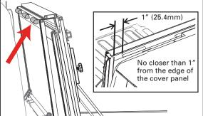
Unfold the cover (A) towards the tailgate. Then confirm each panel is centered side to side and front to back on the truck bed. If adjustments are needed, loosen the cover retainer clamps (E) and shift the cover until positioned correctly. The rear edge of the cover and tailgate seal should rest on top of the tailgate. For proper sealing, the tail panel will overlap by .5".
