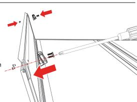
9 Set the cover (A) in the folded position on the side rails (B & C) towards the cab of the truck. Confirm the cover is evenly spaced between the rails.
