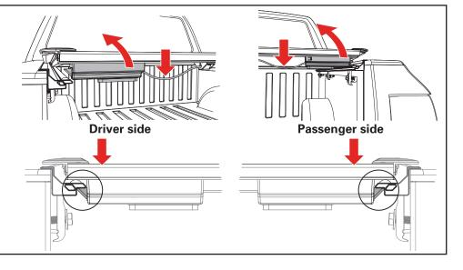
Retighten the cover retainer clamps once the desired fitment is reached. You are ready to drive with your cover in the closed position.
