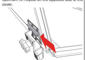
First, prep the buckle ends (F) by peeling off the adhesive liner of the gasket (G).
