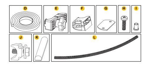
Installing Bulkhead Seal: Clean the top of the bulkhead with soap and water to remove dirt and debris. Clean the area with isopropyl alcohol to remove wax or grease and to evaporate any remaining water. Allow the surface to dry. Peel the backing and adhere the seal (D) from one bulkhead edge to the other. Remove any excess with scissors or a utility knife. Apply pressure evenly to the entire seal to ensure proper adhesion. If the truck has a drop-in bedliner, no seal will be needed.
