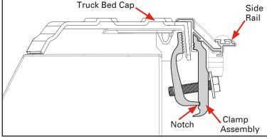
Before placing the cover (C) onto the vehicle, slide two cover retainer clamps (F) into the track on the underside of the cover (C) near the cab. Confirm the cover retainer clamps fit properly into the cover rail for optimum fit. Repeat on the opposite side of the cover.
