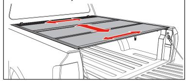
Check if the latches are hitting or not engaging the side rails (A & B) by releasing each latch. If any of the latches need modifications refer to the Slam Latch Adjustment section on the next page on how to make adjustments.
