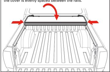
Confirm the retainer clamps (F) are positioned around the side rails (A & B) correctly as shown below. Tighten the retainer clamps by turning them clockwise until the lock washer is secure.
