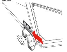
First, prep the buckle ends (H) by peeling off the adhesive liner of the gasket (K).
