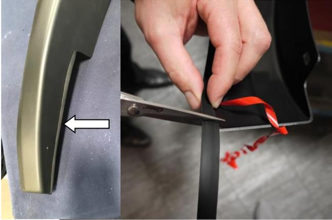
**STEP 3:** Attach rubber seal to the bottom front corner of front and rear Fender Flares per the attached image that will locate around the factory spats. Trim any excess gasket and discard.
