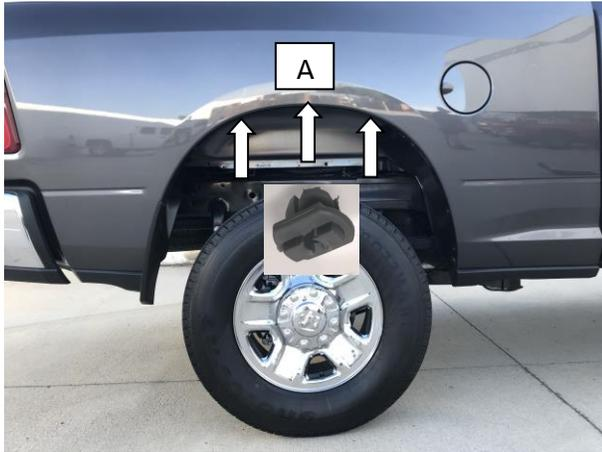
**STEP 10:** Insert grey screw plug into vacant holes at position (A) ensuring that the raised head of the screw plug runs parallel with vehicle body.
