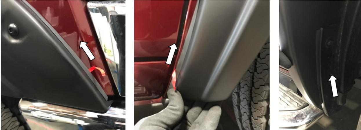
**STEP 7:** Starting at the front of the Fender Flare, carefully remove tape liner from rubber gasket a few inches at a time. Ensure rubber gasket is not tucking into flare and sits flush neatly against the fender body. Ensure all fixing points are tight and secure. Apply forward pressure to adhere the gasket along the edge of entire length of Fender Flare once gasket liner is removed. Repeat install steps for the opposite side of the Fender Flares.
