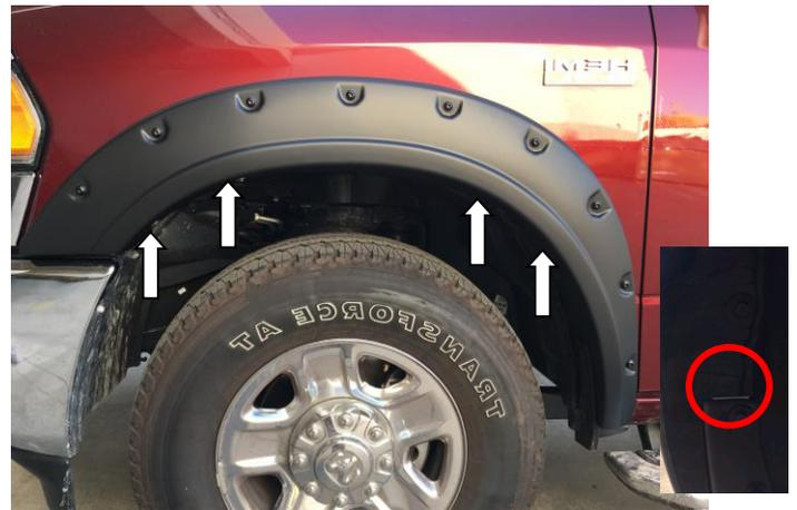
**STEP 6:** Using the previously removed hex head screws, loosely install flares beginning at the front of the flare working to rear. Ensure the cut-out shape fits around factory mud spat against vehicle surface. Ensure the previously removed one inch of tape liner from front and rear Fender Flares is on the outside of the rubber gasket. When satisfied with position, completely secure the (4) hex screws.
