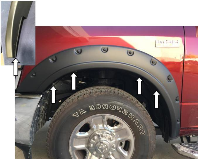
**STEP 5:** Hold Fender Flare towards vehicle in the position of best fit. Note the (4) slots in the flare that correspond with factory installed hex screws in the wheel arch. Remove factory hex screws and retain for later re-installation. Peel back one inch of tape liner for the rubber gasket each end of the Fender Flares then fold at 45 degrees outside of the Fender Flare. Remove one inch of tape liner from the rubber gasket that locates around the factory spat.
