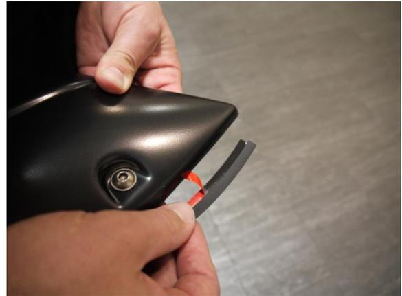
**STEP 2:** Attach the included gasket to the Fender Flares. Peel back 2" of the adhesive backing and position on the Fender Flare. Attach the gasket to the Fender Flare, peeling back a few inches at a time. Ensure pressure is used to secure gasket to Fender Flare edge. Attach gasket along all areas the Fender Flare will make contact with the vehicle body.
