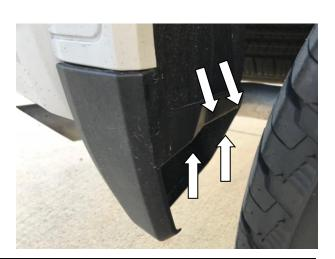
**STEP 11:** Using #15 Torx head screwdriver remove the two upper and two underside screws from the rear factory mud guards in the rear wheel arch. Fender flares require the rear mud guards to be removed, maintain screws for re-install if required.
