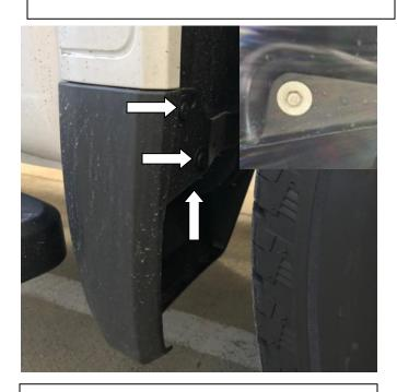
**STEP 5:** Using #15 Torx head screwdriver remove the upper and lower screws from the front factory mudguards and using M10 socket remove the underside screw indicated above, maintain #15 Torx head screws for reinstall . Fender flares require the mud guards to be removed. Retain factory mudguards for later use if required.
