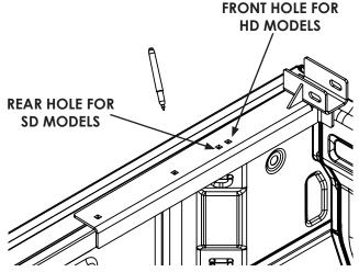
\*\*USE EXTREME CAUTION WHEN DRILLING\*\* Improper drilling can cause damage to your
