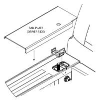
For the 30221 kit place rail plate over the stake pocket bolt and position notch against the front of the bed as shown
