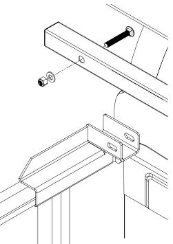
Fasten the RealTruck Backrack to the Rail mount bracket, or Toolbox bracket. Finger tighten at this stage. Center rack on truck and fully tighten both carriage bolts, and 3/8" rail mount bolts. Tighten 3/8" nut to secure.
