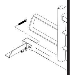
Fasten RealTruck Backrack Assembly to the Stake pocket bolt as shown. Center the RealTruck Backrack assembly on the truck and inal torque all bolts starting with the nuts on the inside of the truck bed, then the rail mount bracket and inally the main RealTruck Backrack carriage bolt.
