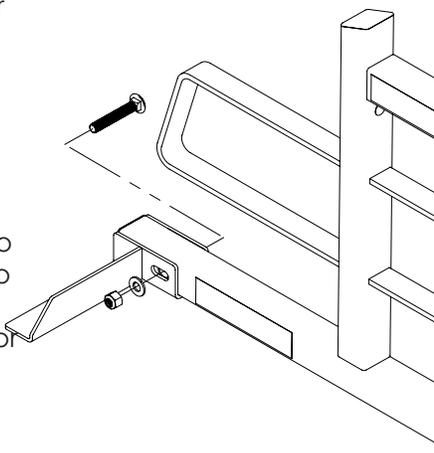
Fasten RealTruck Backrack Assembly to the Stake pocket bolt as shown. Center the RealTruck Backrack assembly on the truck and final torque all bolts starting with the nuts on the inside of the truck bed, then the rail mount bracket and finally the main RealTruck Backrack carriage bolt.
