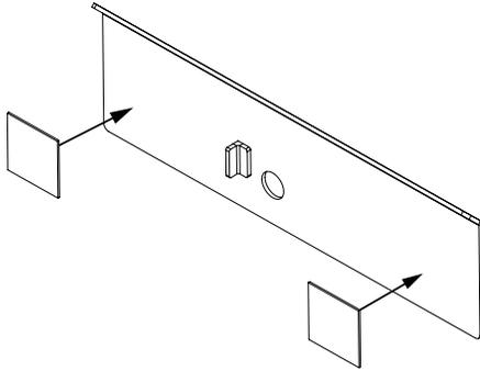
Apply single sided adhesive pads to this side of spacer.
