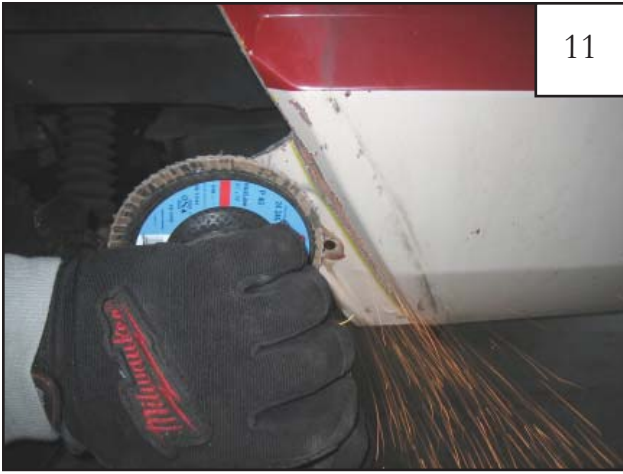
Along rear fender well edge, take care not to cut through weld seam. Cut close to seam, then grind back.
