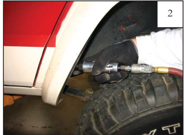
Using a 10mm socket, remove the factory fastener located inside the front of the wheel well.
