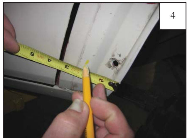
At bottom front of wheel well opening, measure in 2" and make a mark using a grease pencil.
