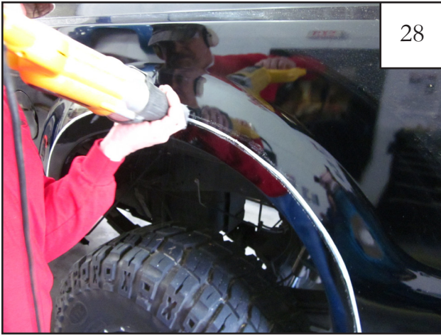
Using a sawsall, cut along inner edge of tape line. WARNING: Angle blade downward/inward for a better (angled) cut in the double walled sheet metal and to avoid cutting support rod . See next step.
