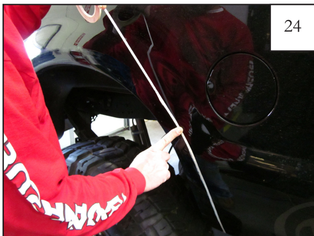
Using marks as a guide, use masking tape to create an arc from the lower mark to the upper mark, then continue around wheel well along style line. See Step 25.
