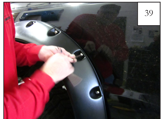
Reattach factory support bar bolt, removed in Step 37, through front mounting hole. Using torx bit (SW1-0052), start bolts installed in Step 38 through holes drilled in Step 36. Once all bolts are in place, tighten all screws.
