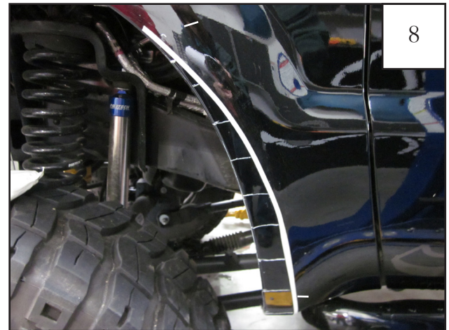
Mark fender with grease pencil about every 2" up to edge of masking tape. NOTE: Ensure sufficient space allowed around pre-existing holes to maintain hole integrity.
