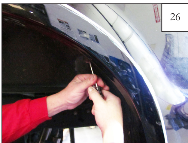
Using a pry tool, remove two factory installed tufflocs from splash guard
