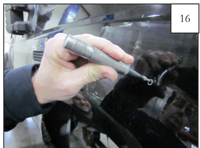
Remove screws installed in Step 14 and flare. Using marks made with scratch awl as a guide, use a center punch to score sheet metal prior to drilling.
