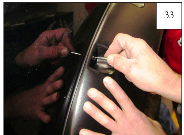
Align fender flare with support bar mount as a reference. With a partner holding flare in place, using a scratch awl and pocket holes in flare as a guide, mark vehicle for drilling.
