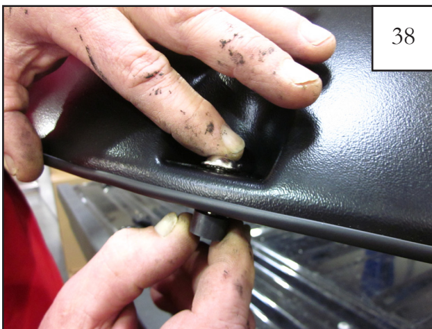
Thread bolt (SW1-0045) through pocket hole in flare then install spacer (SP1-0009) over end of bolt. Hand tighten spacer on bolt until snug near flare plastic. For rear mounting bolt use (SW1-0056) and space (SP1-0009).
