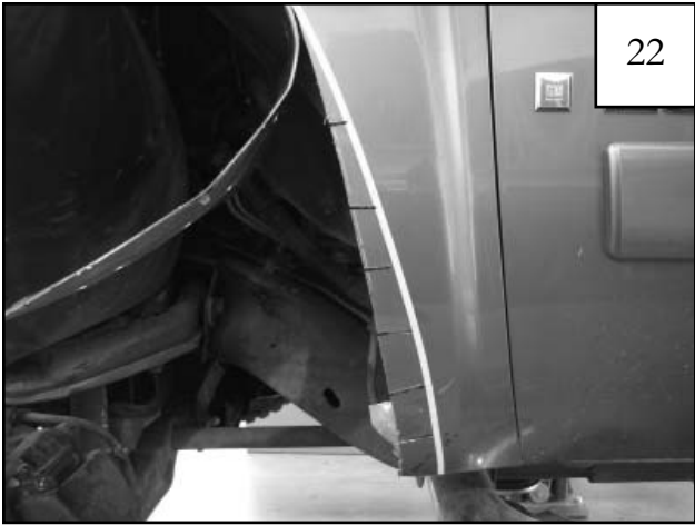
Cut fender approximately every 2" up to edge of masking tape.
