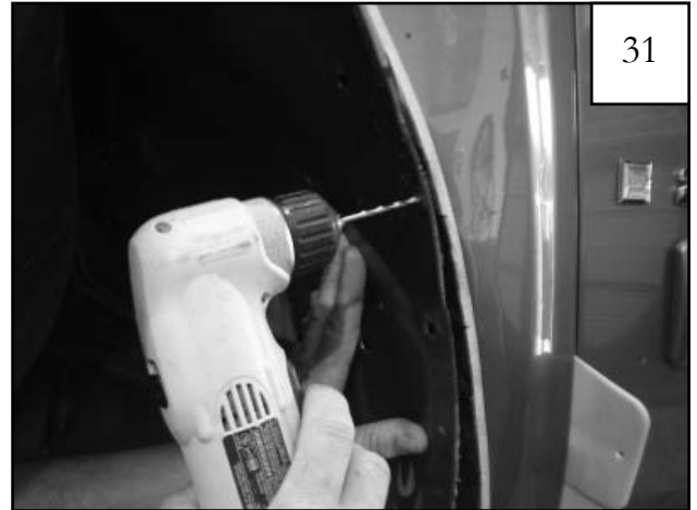
31 With 3/32" drill bit, drill through mark and the bent tabs of metal behind them for three locations along edge of wheel well.
