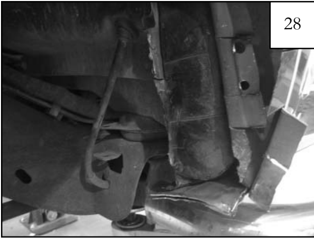
28 Cut pinch seam at mark made in previous step. Bend flange back even with firewall.
