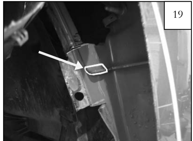
Cut off outlined tab to make bend in the next step easier.
