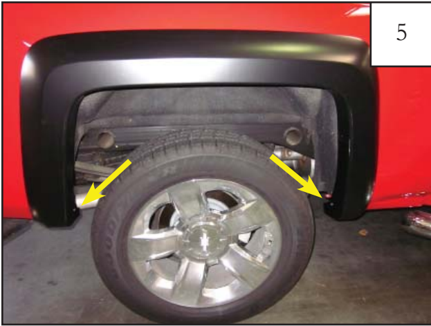
Hold flare firmly in place on fender. Start supplied screw (SW1-0056) at bottom most screw locations (shown). DO NOT TIGHTEN.
