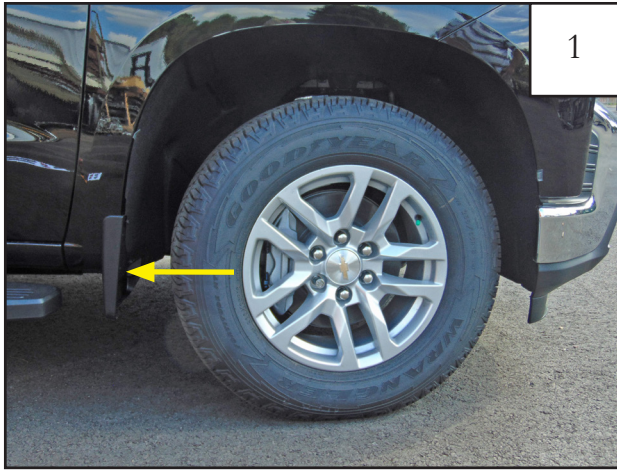
Locate the factory installed mud flap on the passenger side front wheel well.
