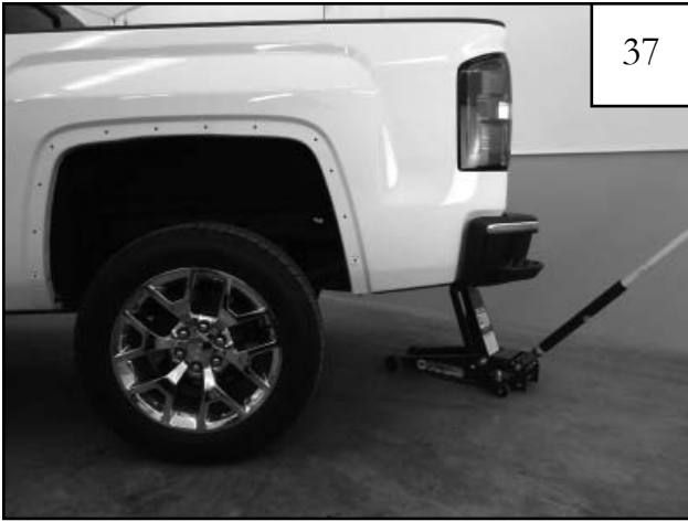
Rear fender/truck bed must be raised to gain access for drilling. Use a floor jack on the rear hitch to raise the truck bed, or remove the rear tire to allow clearance for drilling.
