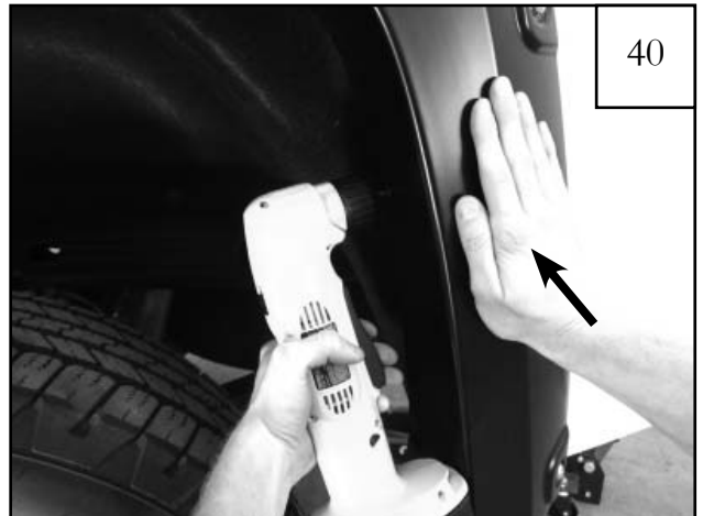
Install self-tapping screws (SW1-0066) into pilot holes drilled in step 36 (3 places). Press flare firmly towards the vehicle while fully tightening.
