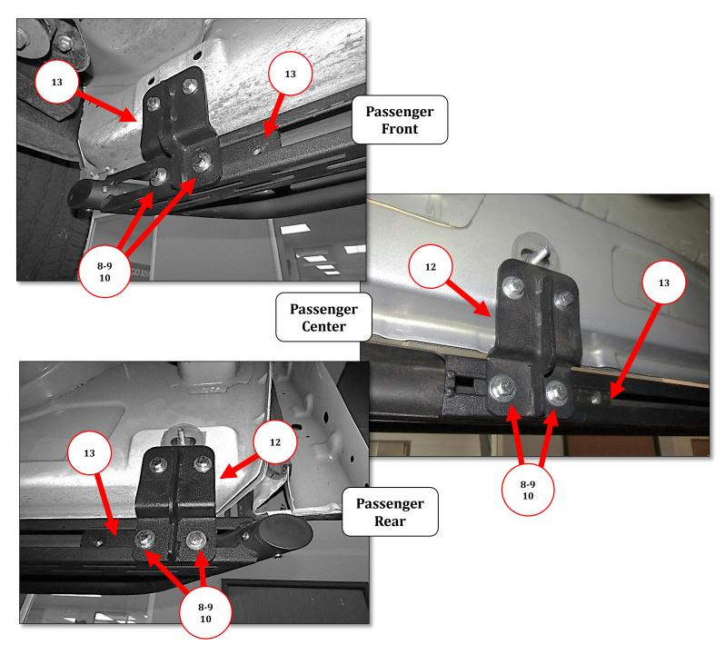
**Step-10** Tighten all bolts securing the Dominator D6 side step to the three side step brackets. Repeat the above steps to install the side step brackets and Dominator D6 side step on the driver side of the vehicle. Remember to check and retighten the nuts and bolts every six months.
