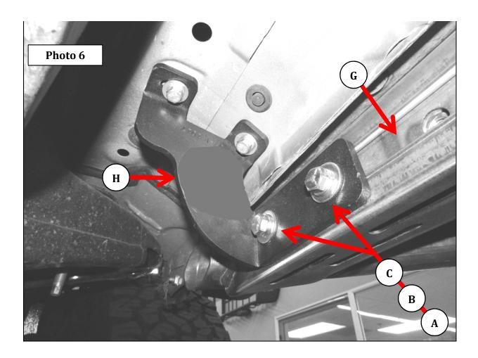
**Step-7** Align the running board with the vehicle and tighten all bracket and side step nuts and bolts,. Repeat the above steps to install the driver side brackets and running board. Remember to check and retighten the nuts and bolts every six months.
