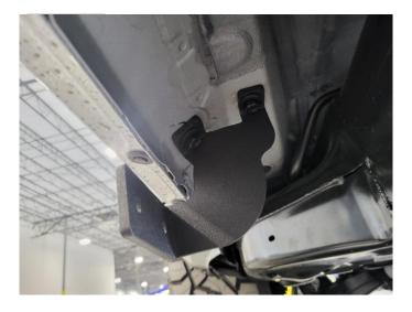
**Step-3** Locate the (2) M8 factory bolts in the underside of the body panel, at the center of the cab (FIGURE 3).
