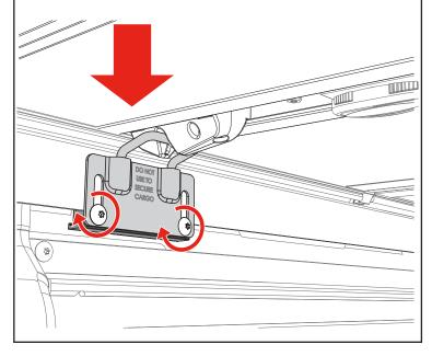
Open the cover by twisting the actuator knob and lifting
