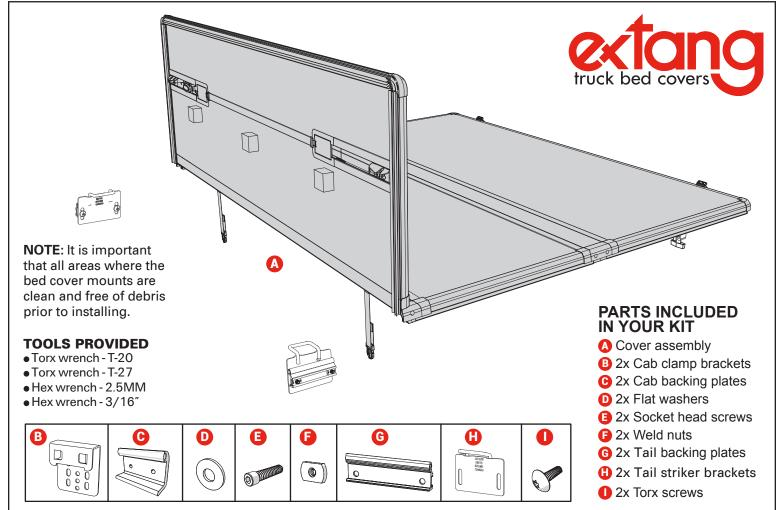
Place the folded, cover on the cab end of the truck bed. Make sure the cover is square with the truck bed and the bulkhead seal sits on the truck bed bulkhead.
