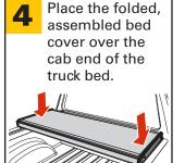
Unfold the bed cover fully and adjust the position over the truck bed for proper front (cab) and rear (tailgate) alignment. When positioned front and back, the tailgate seal should contact the tailgate with the first two fins.
