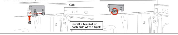
**3** Remove the factory flange bolt, place the rear latch bracket (C) as shown and replace the factory flange bolt along with installing a Torx screw (F). Tighten the factory bolt (T-45) to 16 ft-lbs (22Nm) and the Torx screw (T-30) to 8 ft-lbs (11Nm).
