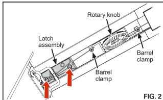
Rotate the rotary knob until you see the flat head screws. Tighten the two screws using the provided Torx T-20 wrench. (Fig. 3)
