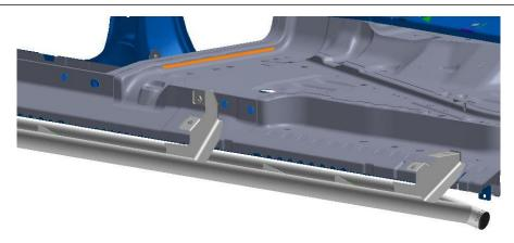
Step 5: Next, tighten the three lower bolts first, following with the three upper bolts.Step 6: Repeat steps 2-5 with passenger side.Step7: Your install is now complete.
