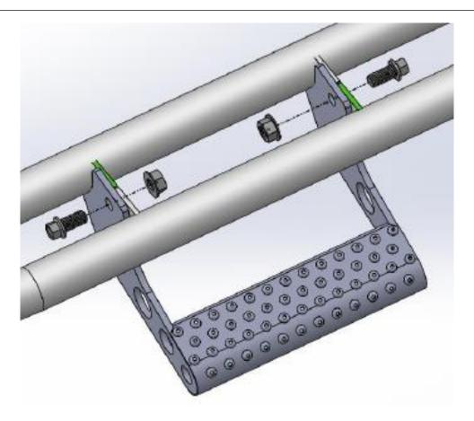
Step 2: Torque bolts to a target of 40 ft/lbs. / 54nm
