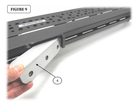
**Step-9** Place and attach the passenger side Dominator running board by each bracket using (2) 3/8" x 1 ¼" hex bolts, (2) 3/8" lock washers, (2) 3/8" flat washers, and (1) 3/8" Nut-Plate (FIGURE 10).
