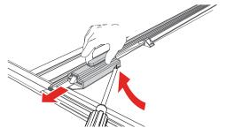
If adjustment is needed, use a straight screwdriver to partially pry open the tab on the latch housing. At the same time slide the housing away from the latch assembly.
