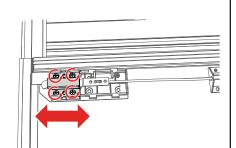
With the latch cover removed, loosen the screws and move the latch bracket to adjust. Re-tighten the screws and slide the latch housing back on.
