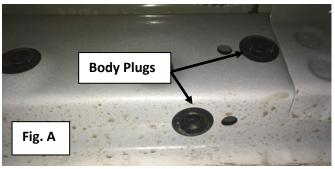
**Step 4:** Using the measurement from the brackets, only remove the rubber plugs from the sections you will need to mount the step. (**NOTE**: *Start with the first section nearest to the front of the vehicle.*)
