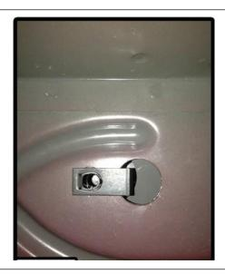
**Step 3:** Install the brackets to the mounting locations in the body of the vehicle and install hardware. Do not tighten all the way.
