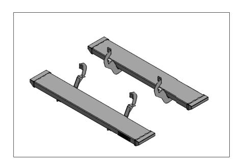
**Step 1**: Look on the underside of the body and locate the factory supplied mounting positions. **NOTE**: Some vehicles require the use of speed clips and nuts, which are supplied with the hardware kit.
