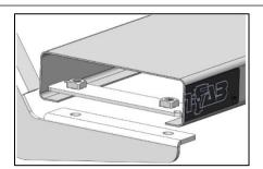
**Step 5:** After final adjustment, tighten (X4) step bolts (25-30 ft/lbs.) and (x4) frame bracket bolts (90-100 ft./lbs)
