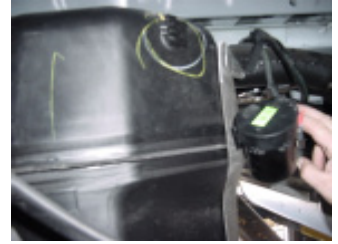
Step 4: Install Turnoverball™ Center Section.
