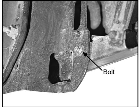
B. Insert bolt through round hole in mounting bracket.
