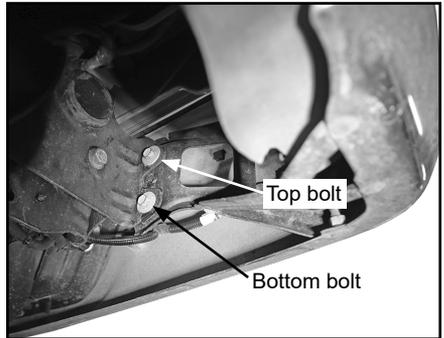
C. Position mounting bracket end with long slot toward inside of box and insert top of mounting bracket under indicated top bolt.
