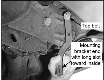
E. Tighten bolts with ratchet and 15 mm socket.
