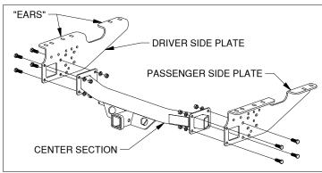
Figure A1: Center Section & Side plates.
