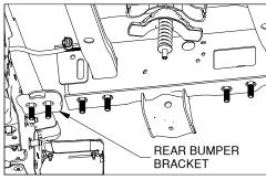
Figure B1: Under Driver side of frame.
